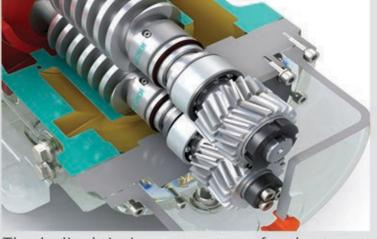
The helical timing gears transfer the torque from one screw to the other with reduced noise.
