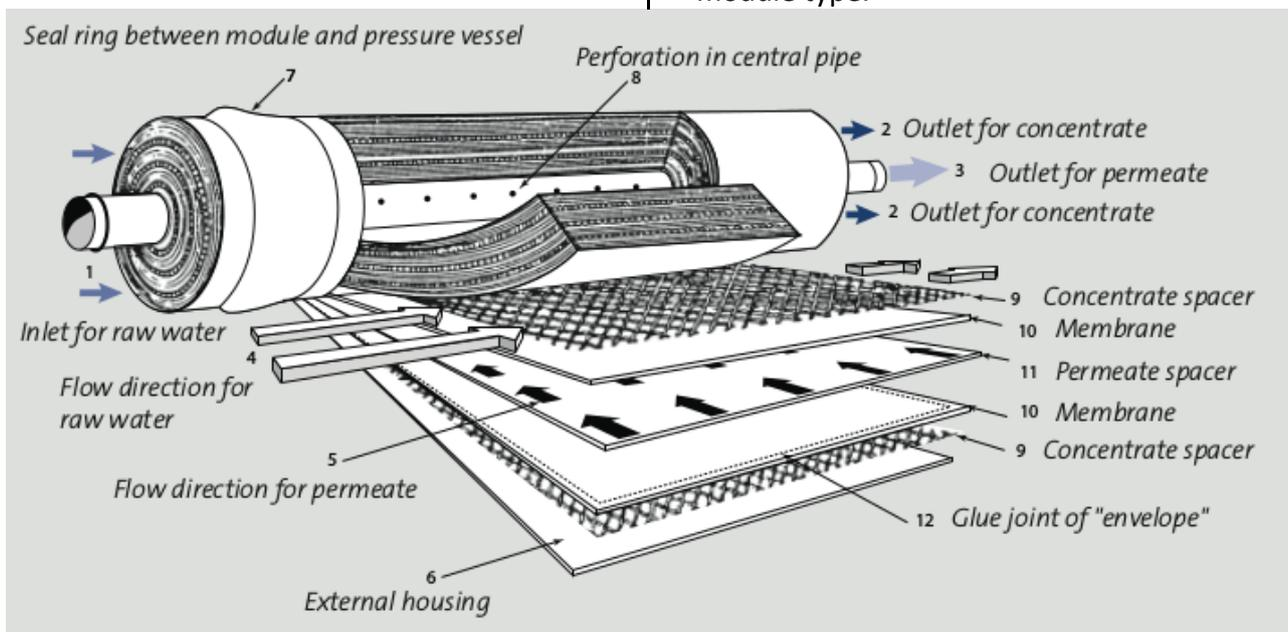
Figure 6 Reverse osmosis: Structure of a spiral wound module
